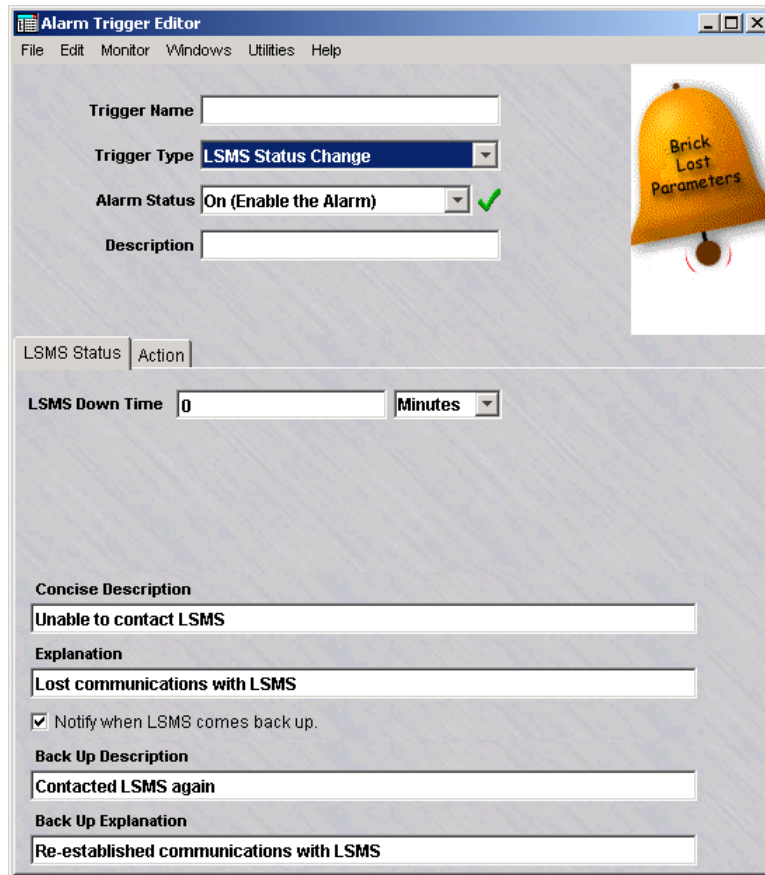
Figure 6-24 Alarm Trigger Editor LSMS Status Change Trigger Parameters
